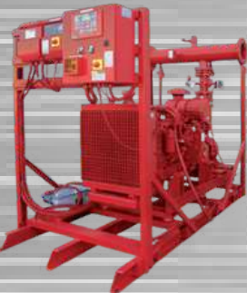
Fire Fighting Units with horizontal pumps back pull-out type, made according to standard EN 12845. Nr. 1 Main Diesel Motor Pump + Nr. 1 Jockey Pump
