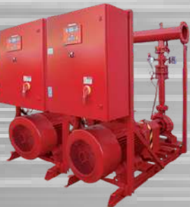
Fire Fighting Units with horizontal pumps back pull-out type, made according to standard EN 12845. Nr. 2 Main Electric Pumps + Nr. 1 Jockey Pump
