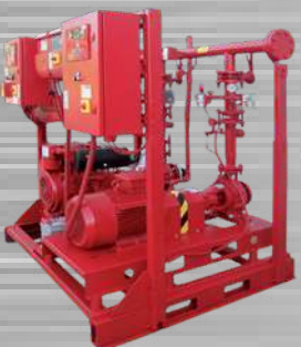
Fire Fighting Units with horizontal pumps back pull-out type, made according to standard EN 12845. Nr. 1 Main Electric Pump + Nr. 1 Main Diesel Pump + Nr. 1 Jockey Pump
